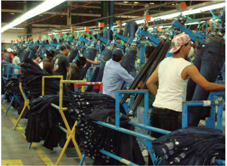
Preparing jeans on mannequins to begin the sanding process.
