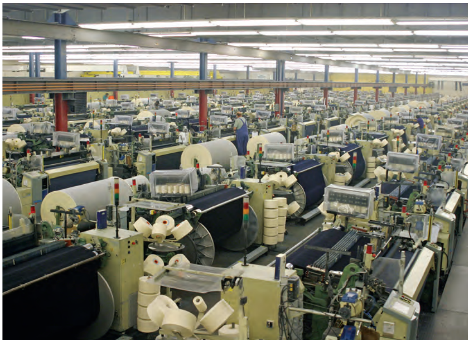
ACG's Weave room includes 161 Air Jet Looms
