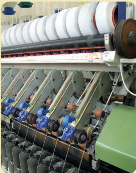
Closer view of spinning frame showing spools of filament entering the draft zone of the spinning frame.
